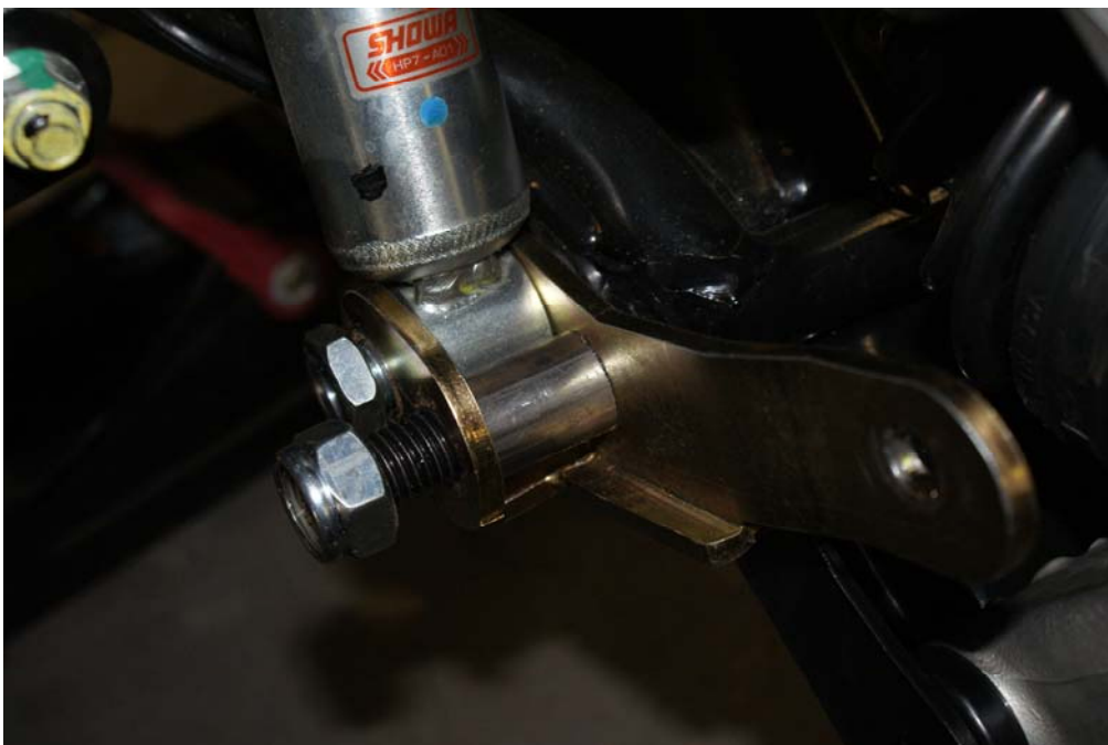
PHOTO #5 view from dr. side Note placement of nuts.
